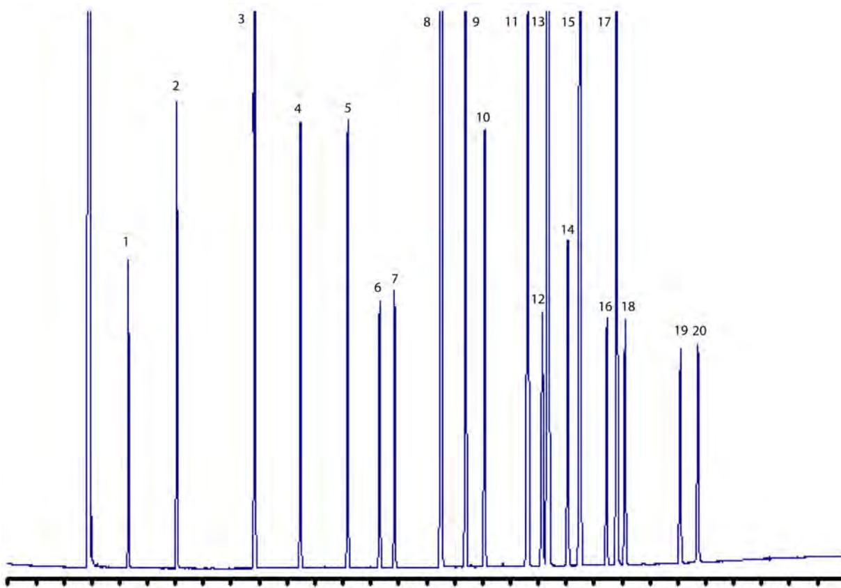
Cat# 4210 spiked with 0.4 mg/ml C18:2t ester (methyl linoelaidate) and chromatographed on a Supelco SP 2330 fused silica column.
